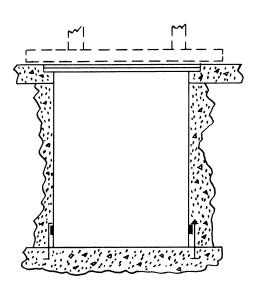
NOTE: Some larger size fiberglass basins are equipped with anchoring ridges near the bottom. Reinforcing rods or threaded bolts and washers may be used to help prevent floatation until the second concrete pour has set.
