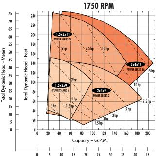
Left hand rotation Certified performance test Packing with lantern ring 250# ANSI B16.1 suction & discharge flanges Water cooled bearing cartridge caps Metallic/Plastic hi-temp packing Stuffing box bushings
